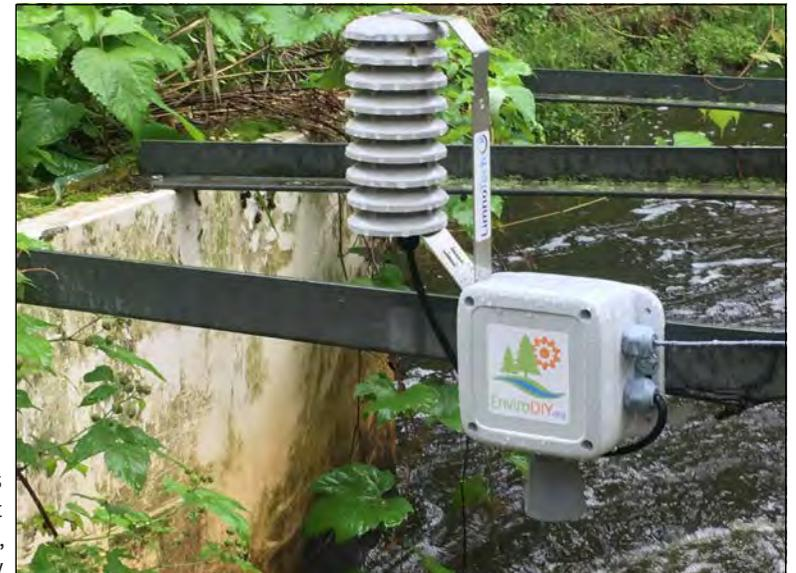
Remote sensors are positioned at Whitaker Pond, Oakmede, County Road F, and Kohler Road, fastened to existing creek flume structures. VLAWMO staff assembled the sensors with the help of EnvironDIY staff.
