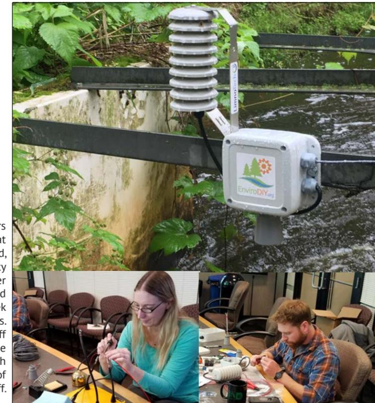
Remote sensors are positioned at Whitaker Pond, Oakmede, County Road F, and Kohler Road, fastened to existing creek flume structures. VLAWMO staff assembled the sensors with the help of EnvironDIY staff.
