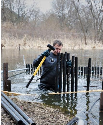
Emil Kukulski, director of Poland-based ProCom System's hydro-ecological department, was on site for a week to test the electrical guidance system. It was developed to keep native fish out of hydroelectric plants' water intake systems. In Michigan, it was adapted to control invasive sea lampreys.
