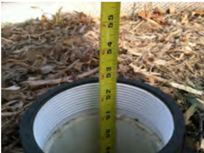
Measurements of sediment build up of the three northernmost access ports to be done on a frequent basis. There will be some margin of error (0.5") due to the rock base but accuracy to determine whether JetVac of the system needs to happen with sediment buildup. The measurement should be noted with the top of the pipe - in this photo the reading is 52-10/16". See Appendix C\_2 for the Inspection Maintenance Report Form.
