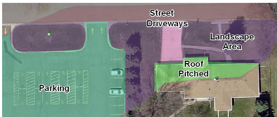
Figure 3. An example neighborhood and the source areas that are entered in to WinSLAMM
