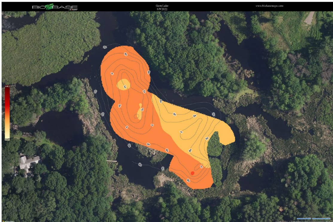
Figure 10. South Gem Lake bottom composition values with 0.3-m contours taken on August 9, 2022.
