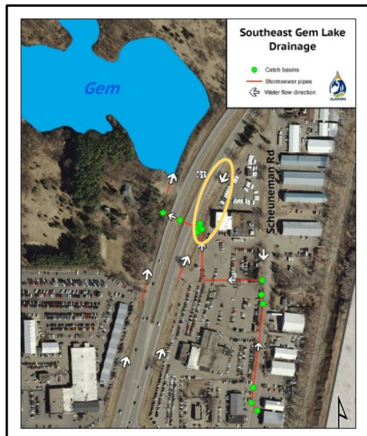
Figure 1: Stormwater swale and catch basins treating stormwater from Hwy 61. This was included in the VLAWMO press release in 2018 announcing the delisting of Gem Lake.
