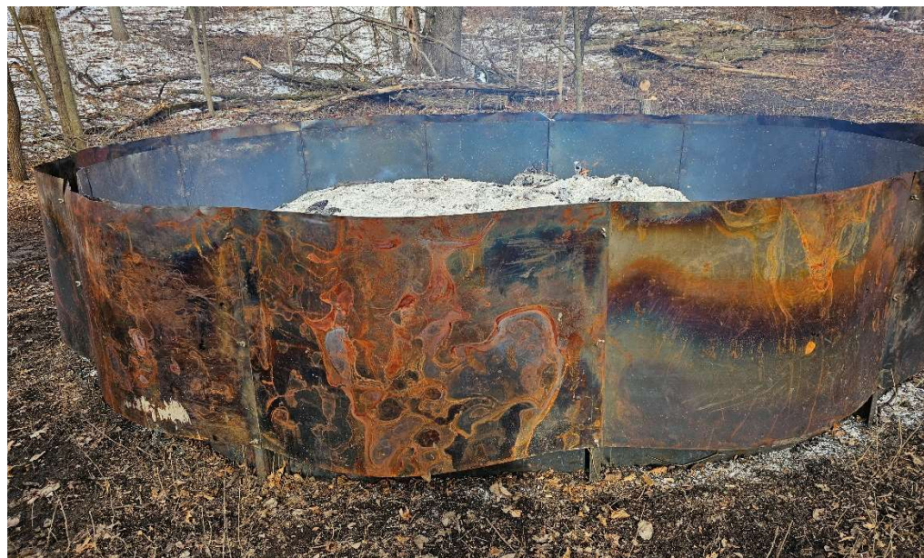
Kiln set-up at Battle Creek Regional Park; kiln is double-sided so that it is insulated by warmed air
