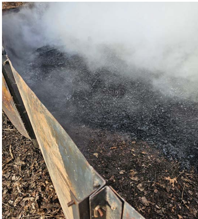
Finished biochar at the end of the firing in the kiln
