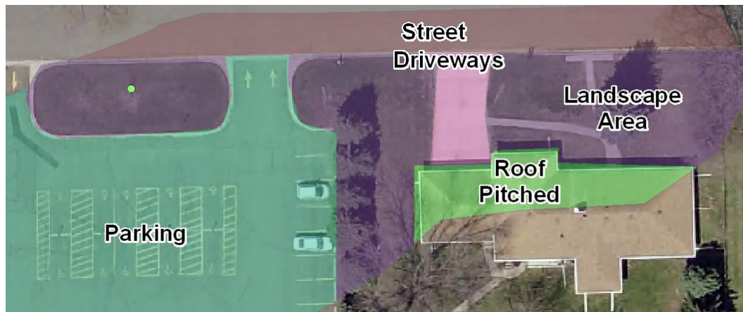
Figure 2. An example neighborhood and the source areas that are entered in to WinSLAMM
