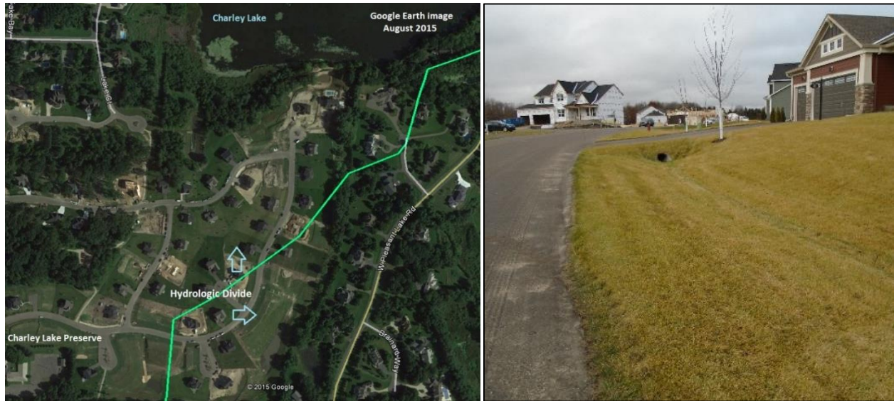
Figure 11. (Left) Charley Lake Preserve’s hydrologic divide between runoff flowing southeast toward Pleasant Catchment and the 28.5 acres of urban runoff flowing north toward the Charley Stormwater Pond. (Right) A typical mowed turf-lined ditch in the Charley Lake Preserve housing development.
