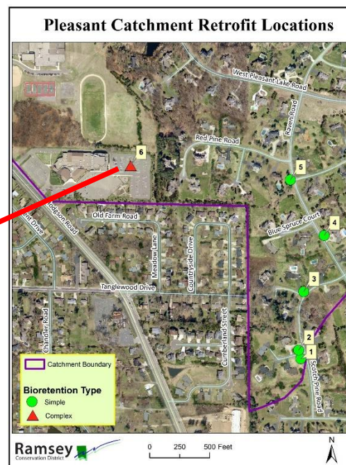
Figure 20. Flooding at Site 6 (left) in the Pleasant catchment (August 2015), Incarnation Lutheran Church parking lot. The proposed BMP involves removing some parking spaces to expand the vegetated area, creating a raingarden to which most of the back parking lot drains. (Right). Map of bioretention sites 1-6, Pleasant Catchment.
