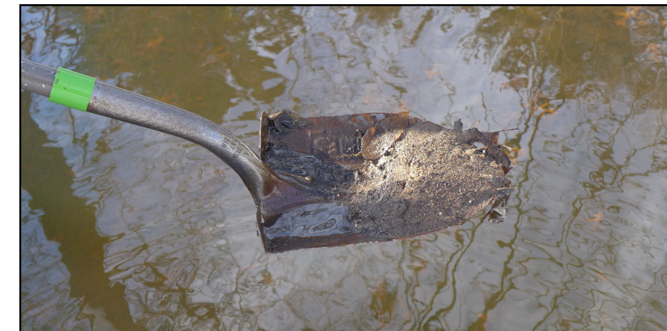
To monitor sediment levels, sediment was scooped with a shovel from the bottom of Lambert Creek and brought to a lab for testing.
