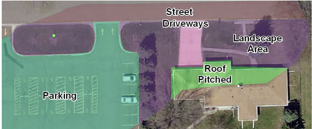
Figure 2. An example of a neighborhoodshed and the source areas that are entered into WinSLAMM (RCD, 2013, p. 7)
